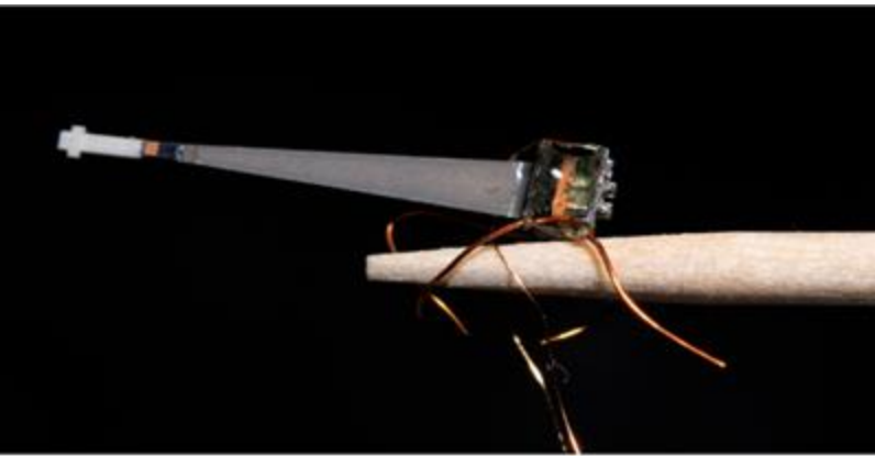
Prototype of a robo-buzzer capable of shaking the stamens of a buzz pollinated plant and releasing pollen. The prototype is attached to a toothpick (2mm diameter) using orange wire "legs" for illustration. CREDIT: Marco Vallego-Marin
